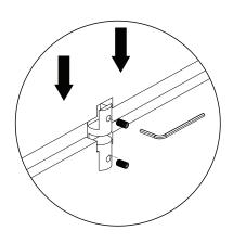
Attach the CVD Clamps between the top panel and bottom panel using the set screw supplied with CVD Clamps
